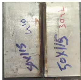
fig 2 Sample of ss304L&ss410 with double v-joint
